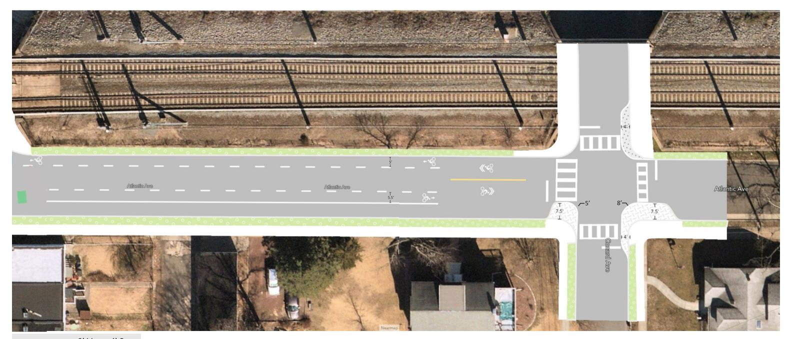
Bike Lane Striping: 3' Line & 4' Gap North Bike Lane Width: 5' South Bike Lane Width: 5.5'
