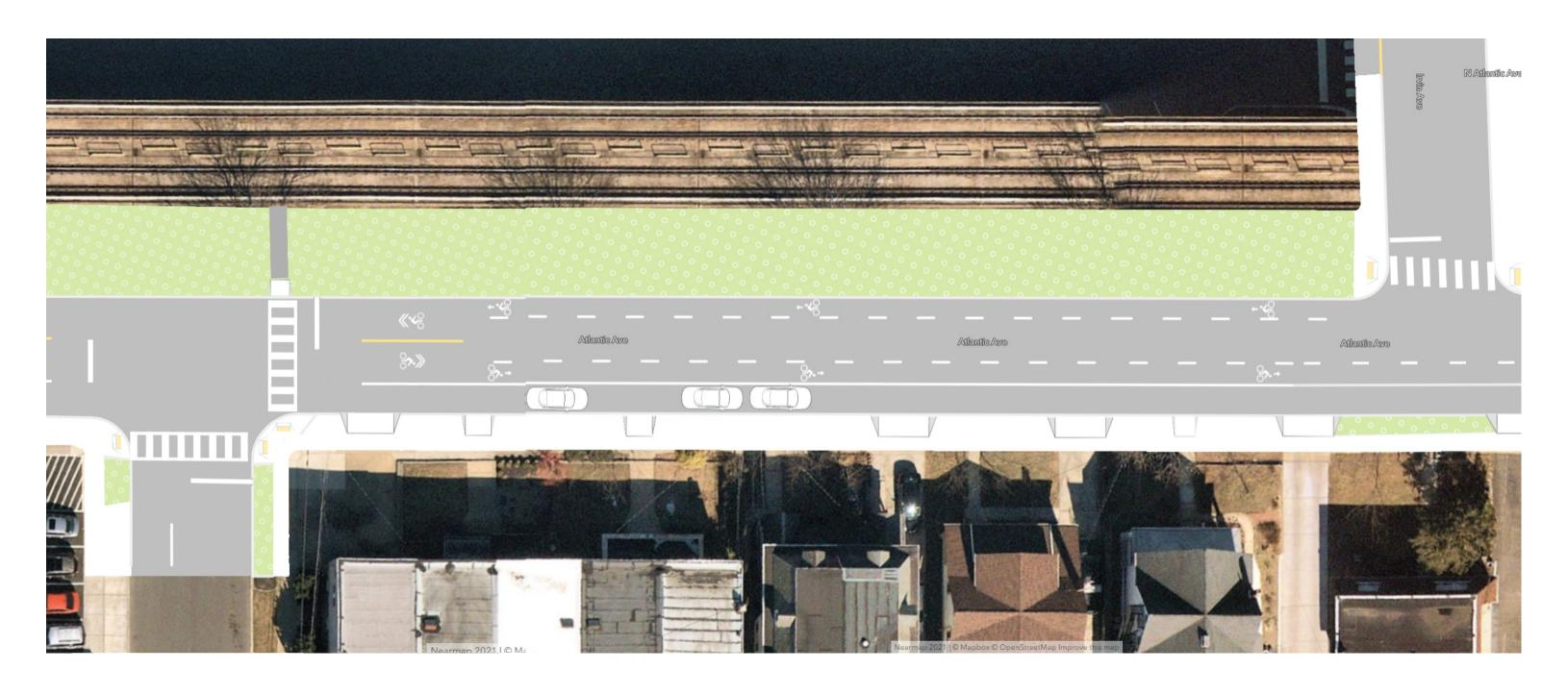
Bike Lane Striping: 3' Line & 4' Gap North Bike Lane Width: 5' South Bike Lane Width: 5.5'
